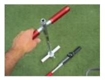
**Step 6** Remove torque wrench from tool.
